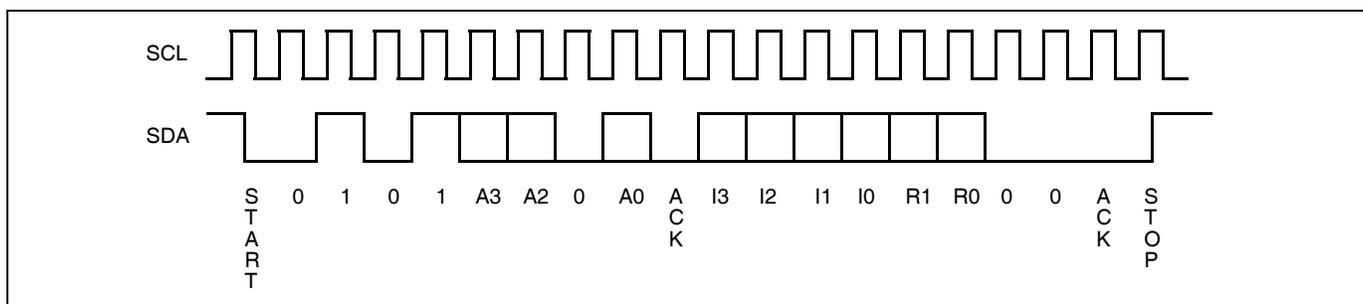
The Increment/Decrement command is different from the other commands. Once the command is issued and the X9428 has responded with an acknowledge, the master can clock the selected wiper up and/or down in one segment steps; thereby, providing a fine tuning capability to the host. For each SCL clock pulse ( $t_{HIGH}$ ) while SDA is HIGH, the selected wiper will
