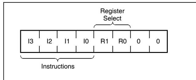
The four high order bits define the instruction. The next two bits (R1 and R0) select one of the four registers that is to be acted upon when a register oriented instruction is issued. Bits 0 and 1 are defined to be 0.
