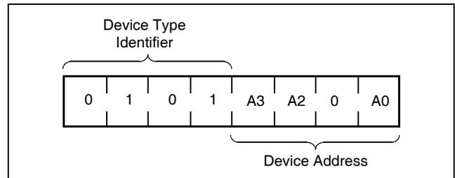
The next four bits of the slave address are the device address. The physical device address is defined by the state of the  $A_0$ ,  $A_2$ ,  $A_3$  inputs. The X9428 compares the serial data stream with the address input state; a successful compare of all four address bits is required for the X9428 to respond with an acknowledge. The  $A_0$ ,  $A_2$ ,  $A_3$  inputs can be actively driven by CMOS input signals or tied to  $V_{CC}$  or  $V_{SS}$ .
