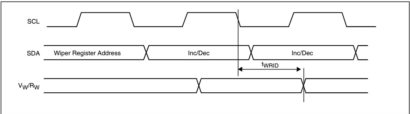
**Write Protect and Device Address Pins Timing**
