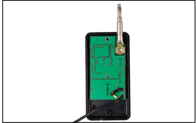
Figure 7. Removing the back cover
