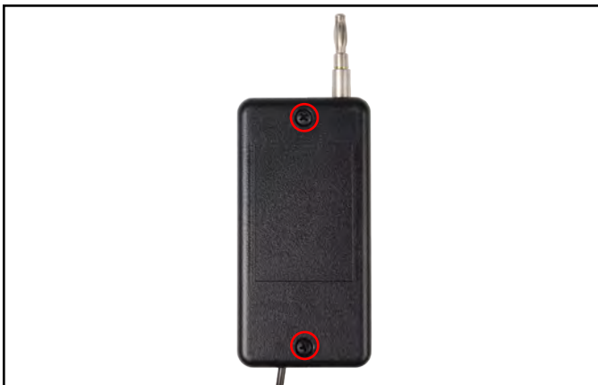
Figure 6. Locating the enclosure screws
