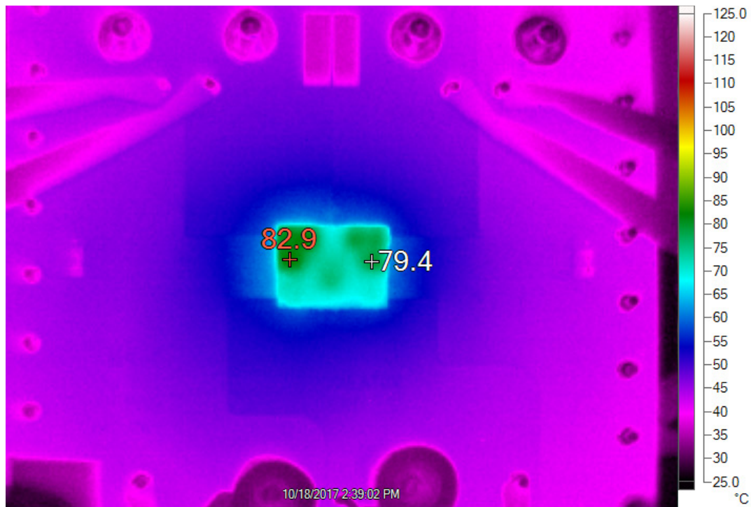
Figure 11. Thermal at V_{IN} = 12V , V_{OUT0} = 1.0V , I_{OUT0} = 10A , V_{OUT1} = 1.8V , I_{OUT1} = 10A , T_A = 25^\circ C , No Airflow
