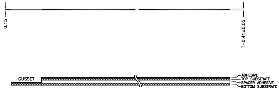
SECTION A-A LAYERS STACK-UP
